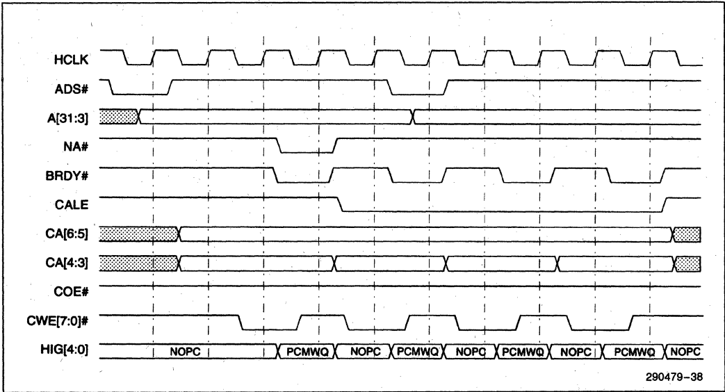
Figure 5-11. Burst Write to Second Level Cache with Standard SRAM
